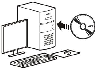
APC PowerChute Personal Edition software provides automatic file saving and shutdown of your computer in the event of a power failure. Use the cable supplied with the Back-UPS to connect the data port on the Back-UPS to the USB port on your computer. Place the CD into your computer, and follow the on-screen instructions.
