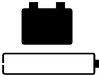
The Back-UPS is operating on battery power and the battery power is getting low. Shut down all connected equipment to avoid losing an unsaved data. When possible, connect the Back-UPS to utility power to recharge the batter.
