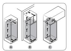
The air outlet must be positioned in one of the examples below, or a similar position, depending on your cabinet type.
