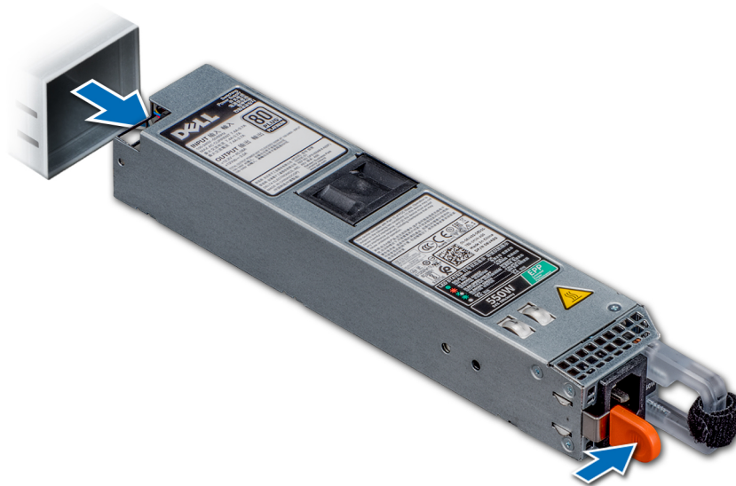
Figure 93. Removing a power supply unit
