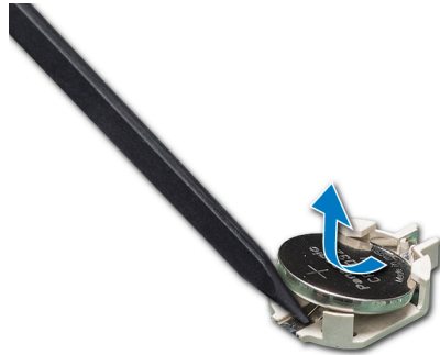
Figure 87. Removing the system battery
