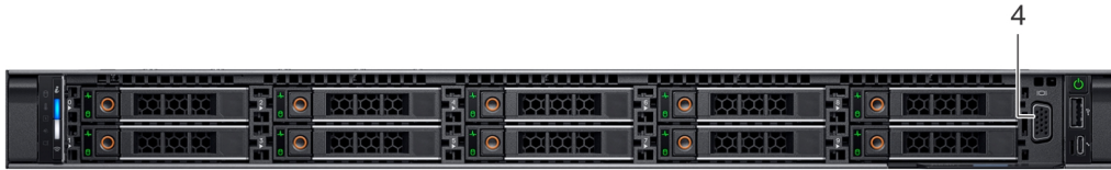
Figure 3. Front view of 10 x 2.5 inch drive system
