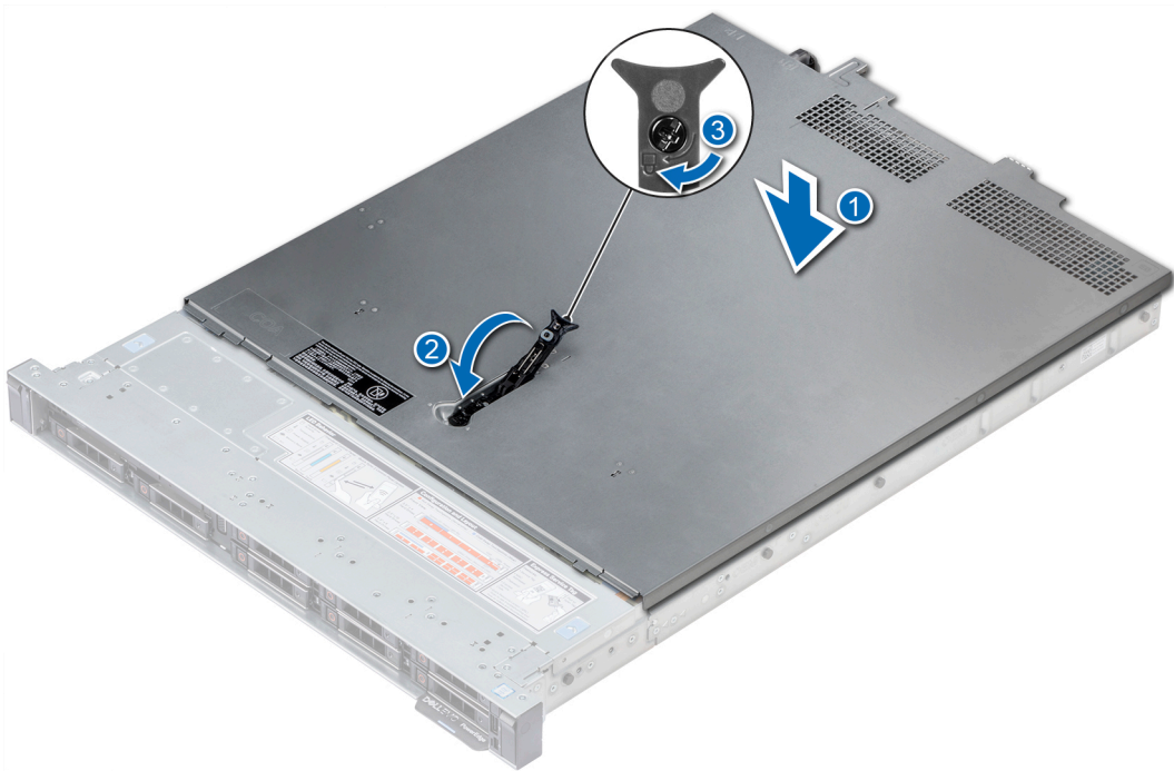
Figure 20. Installing the system cover
