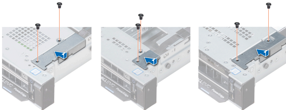
Figure 105. Installing the cable cover
