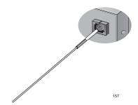
Figure 29. Cleaning a Recessed Ferrule
