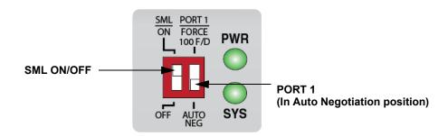
Figure 9. MMC2000/200 Series Converter Rear Panel DIP Switches
