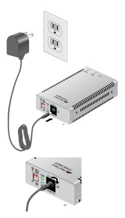
Figure 22. Connecting 12VDC Powered Unit
