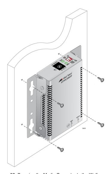
Figure 33. Securing the Media Converter to the Wall
