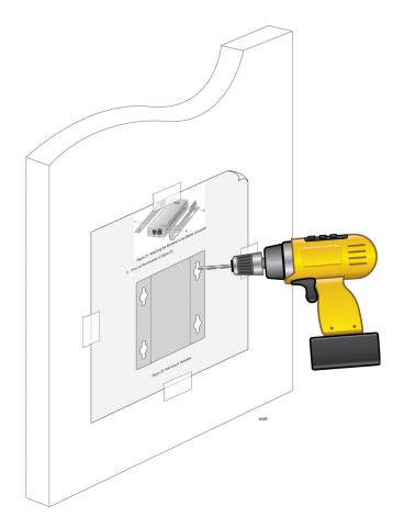
Figure 32. Placing the Template on the Wall
