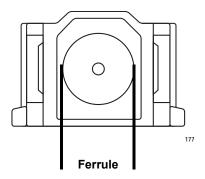
Figure 24. Ferrule in an SC Connector Plug
