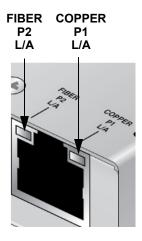
Figure 2. Port LEDs
