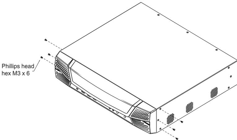
2. Use the M3 x 8 Phillips head hex screws supplied with the rack mount kit to screw the rack mounting brackets into the front of the unit.
