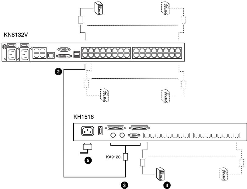
**Note:** The diagram above shows an installation with the KN8132V. Cascading other KN8 Series switches is same as the KN8132V and only differs in that it provides additional KVM ports.
