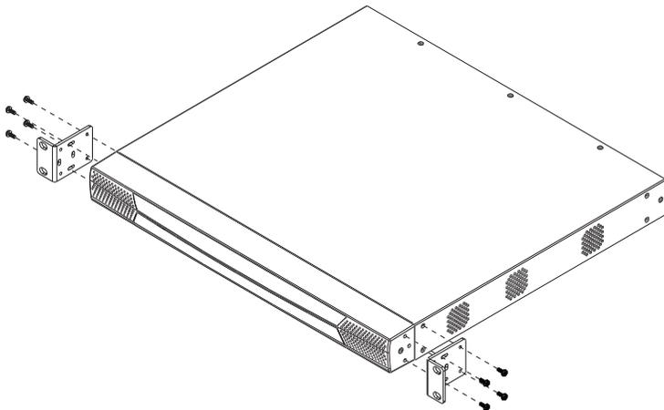
3. Position the device in the front of the rack and align the holes in the mounting brackets with the holes in the rack.
