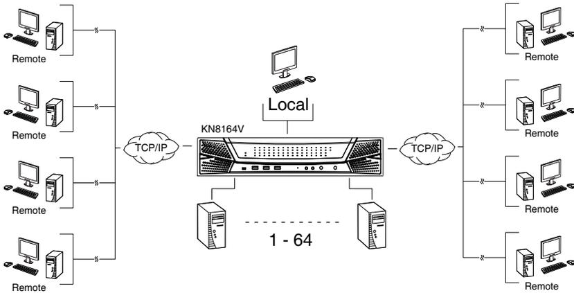
Since the switches use TCP/IP for their communications protocol, they can be accessed via their IP addresses from anywhere on the LAN, WAN, or Internet – whether the connecting computer is located down the hall, down the street, or half-way around the world. Remote operators can log in via their browser or make use of stand-alone Windows or Java GUI applications. Java allows the switches to work with JRE (Java Runtime Environment) enabled operating systems – ensuring multi-platform operability.
