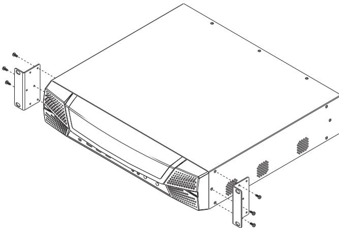
3. Position the device in the front of the rack and align the holes in the mounting brackets with the holes in the rack.
