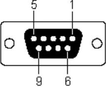
The diagram shows a DB9 Female connector with nine pins. The pins are arranged in a row. The top-left pin is labeled '5', the top-right pin is labeled '1', the bottom-left pin is labeled '9', and the bottom-right pin is labeled '6'. The connector is labeled 'DB9 Female' below it.
