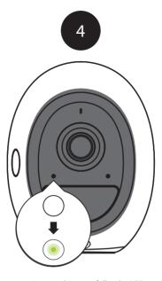
Once at the camera is synced successfully, the LED on the camera will illuminate green to indicate it's currently connected.
