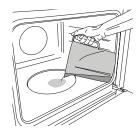
Only when the oven is cold, fill the embossing of the cavity with the quantity of drinking water suggested in the relative cooking table.
