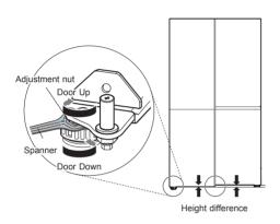
Open the door and use the supplied spanner type 2 to adjust the level of the lower side, using the nut on the adjustable round foot as per the below diagram.
