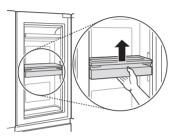
2 To lower moving basket, press up to release the levers at the side of the basket and lower the basket until it clicks into place.
