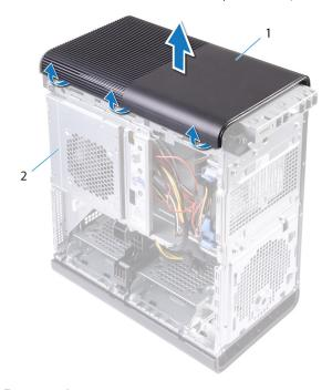
Figure 10. Removing the top cover
