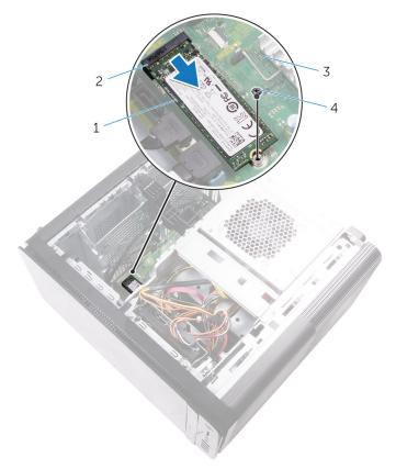
Figure 15. Removing the solid-state drive
