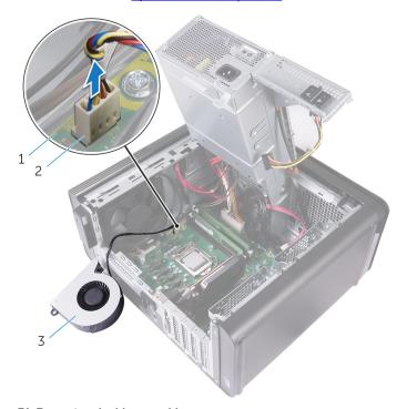
Figure 31. Removing the blower cable
