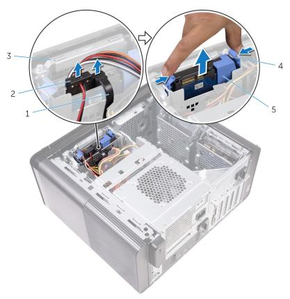
Figure 13. Removing the hard-drive assembly
