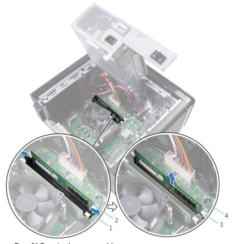
Figure 24. Removing the memory module
