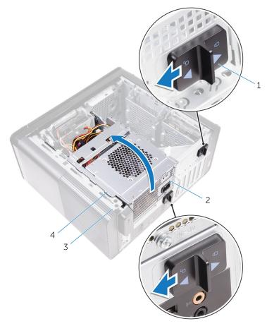
Figure 17. Rotating the power-supply unit
