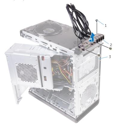
Figure 28. Removing the USB panel
