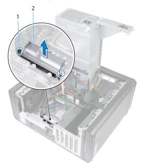
Figure 32. Removing the VR heat sink
