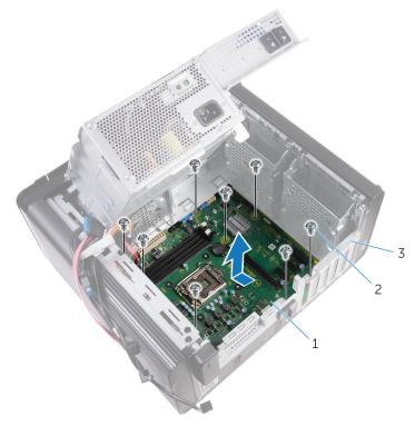
Figure 42. Removing the system board
