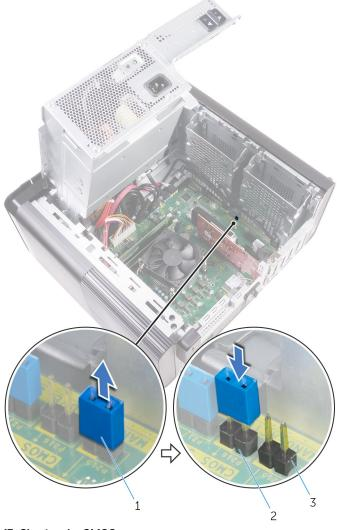
Figure 43. Clearing the CMOS
