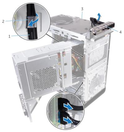
Figure 27. Disconnecting the cables
