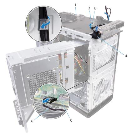
Figure 26. Disconnect the power-button module cable
