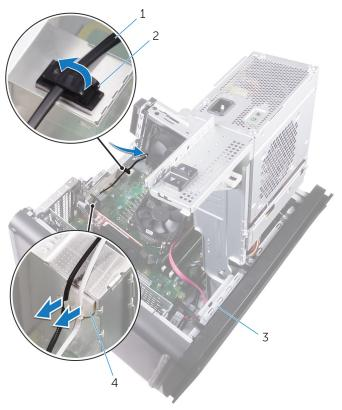
Figure 40. Disconnecting the antenna cables
