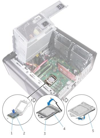
Figure 37. Replacing processor
