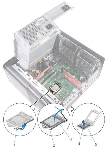
Figure 36. Removing processor
