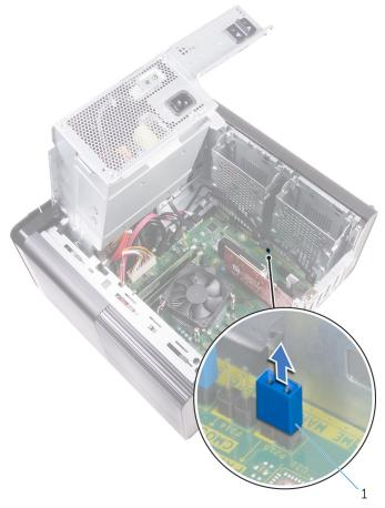
Figure 44. Removing the jumper plug
