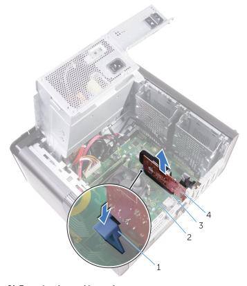
Figure 21. Removing the graphics card
