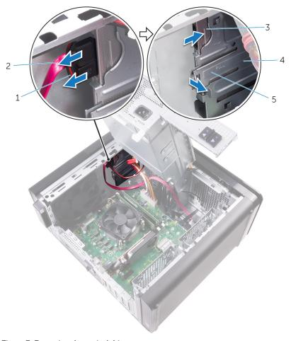
Figure 5. Removing the optical drive
