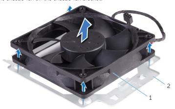
Figure 35. Removing the chassis fan
