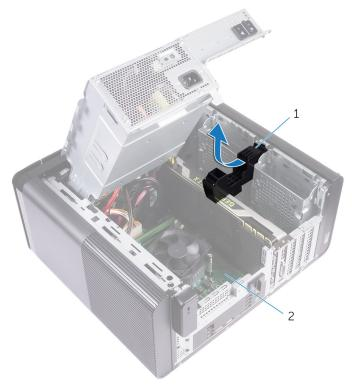
Figure 22. Removing the full-length graphics-card bracket
