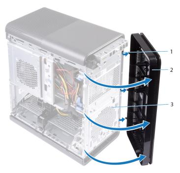
Figure 4. Removing the front bezel
