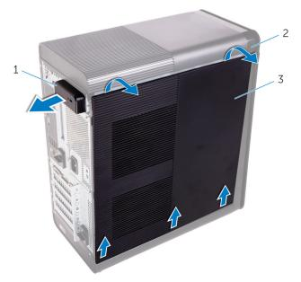
Figure 1. Removing the right-side cover
