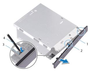
Figure 9. Removing the optical-drive bezel
