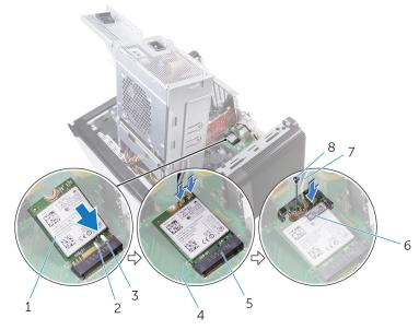
Figure 39. Replacing the wireless card
