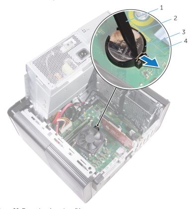
Figure 20. Removing the coin cell battery
