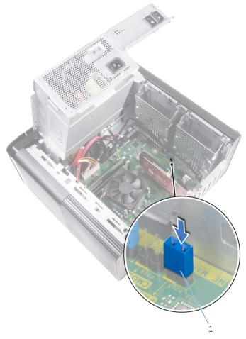
Figure 45. Clearing the password
