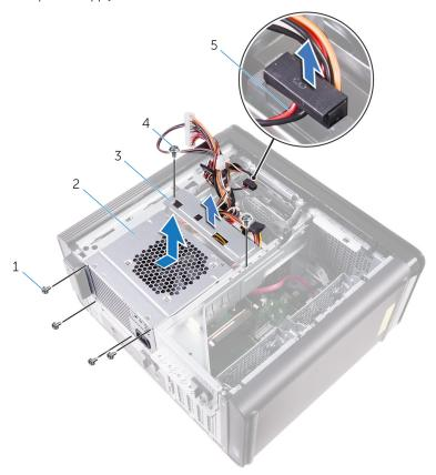
Figure 19. Removing the power supply unit
