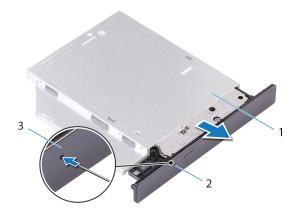
Figure 8. Removing the optical-drive bezel
