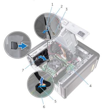
Figure 34. Removing the chassis fan
