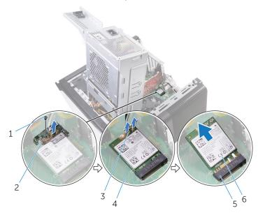
Figure 38. Removing the wireless card
