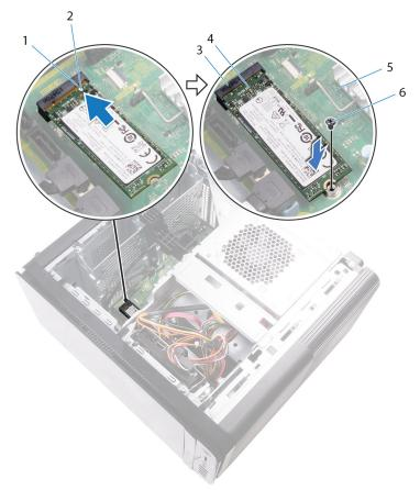
Figure 16. Replacing the solid-state drive
