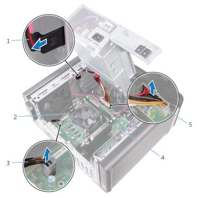
Figure 18. Disconnecting cables
