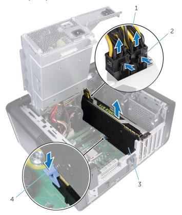
Figure 23. Removing the power cable
