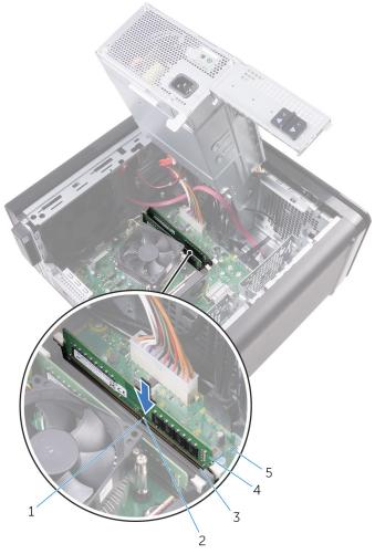
Figure 25. Replacing the memory module
