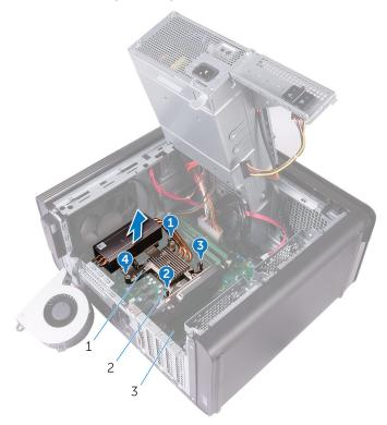
Figure 30. Removing the captive screws
