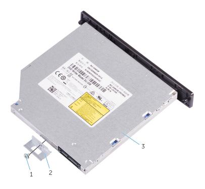
Figure 7. Removing the optical drive
