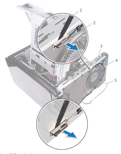
Figure 41. Removing the antenna
