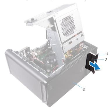
Figure 6. Removing the optical drive
