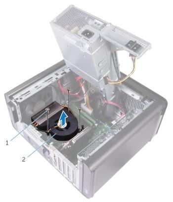
Figure 29. Removing the blower
