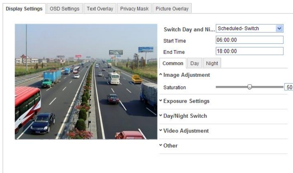
Figure 6-35 Day/Night Scheduled-Switch Configuration Interface
