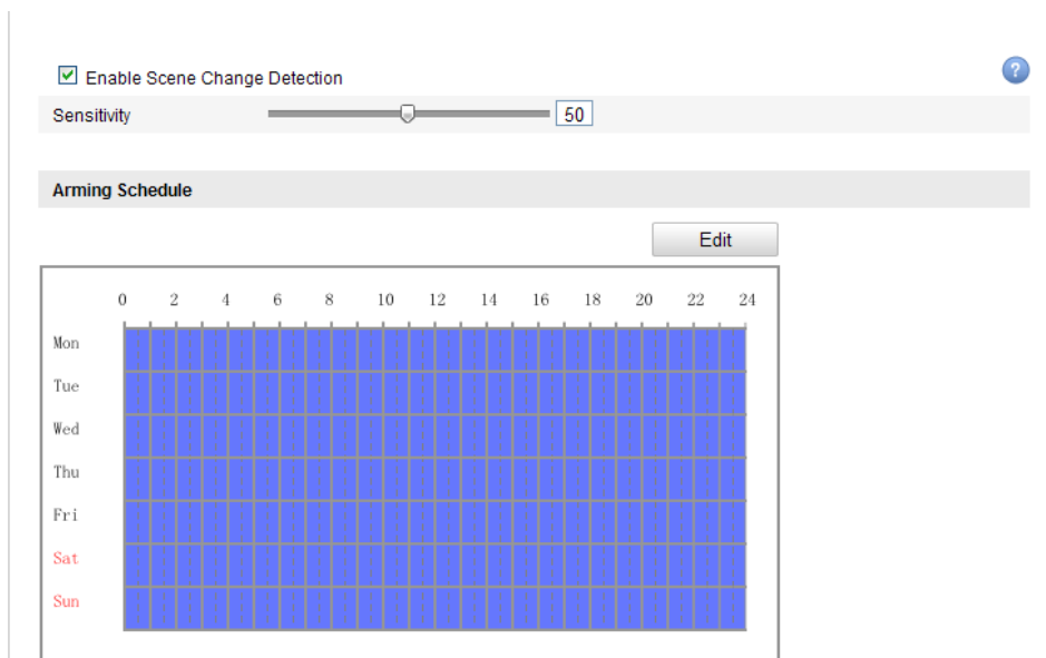
Figure 6-58 Configuring Scene Change Detection
