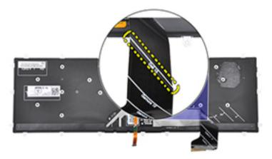
2 Gently fold the keyboard cable with the end aligned at the fold line as shown in the image. Once folded correctly, the right edge of the keyboard cable should be lined up next to the line indicated on the palm-rest assembly.
