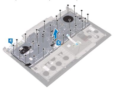
6 Lift the keyboard, along with the cables, off the palm-rest assembly.
