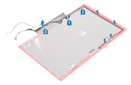
3 After performing the above steps, we are left with the display back-cover and antenna assembly.
