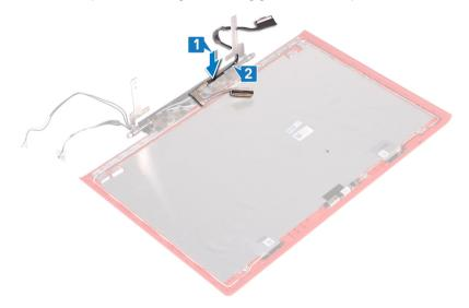
3 Adhere the tape that secures the display cable to the display back-cover and antenna assembly.
