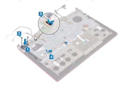
5 Adhere the tape that secures the fingerprint-reader board and the power-button board to the palm-rest assembly.
