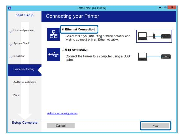
If you connect the printer to the network using an Ethernet cable, the following screen is displayed. Select the printer, and then click **Next**.
