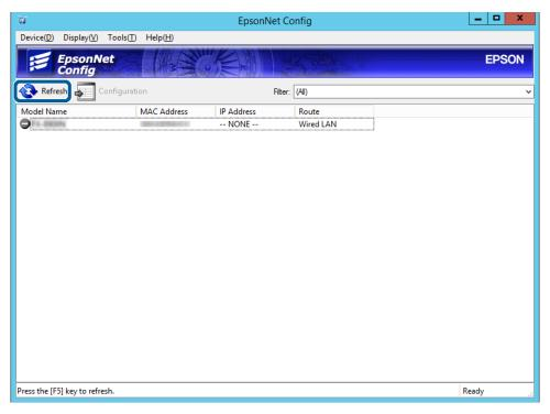
Check that an IP address has been assigned.
