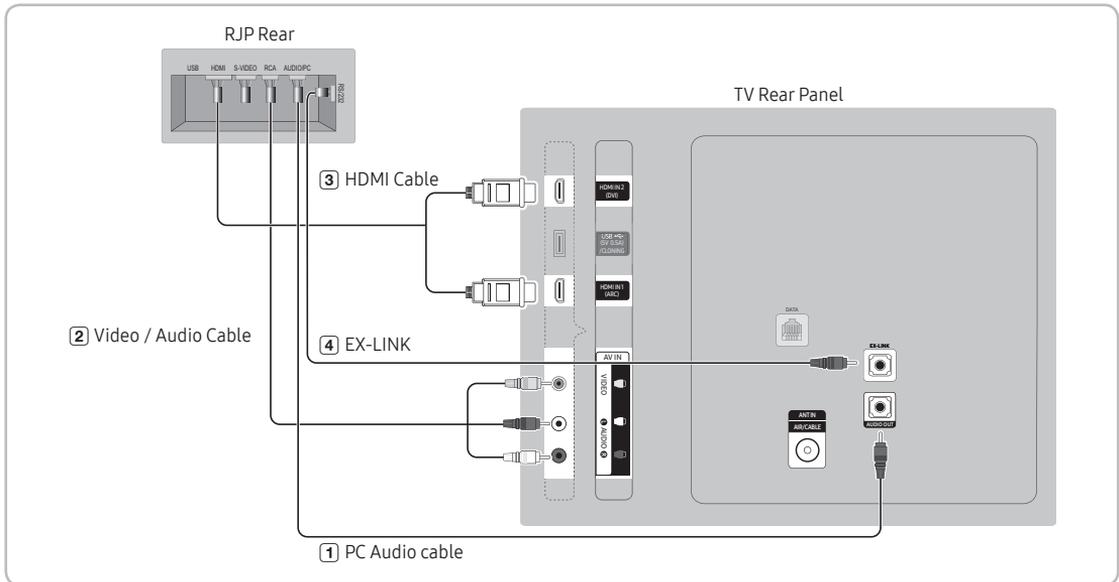
1. Connect the AUDIO OUT port of the TV to the PC/AUDIO port of the RJP.
