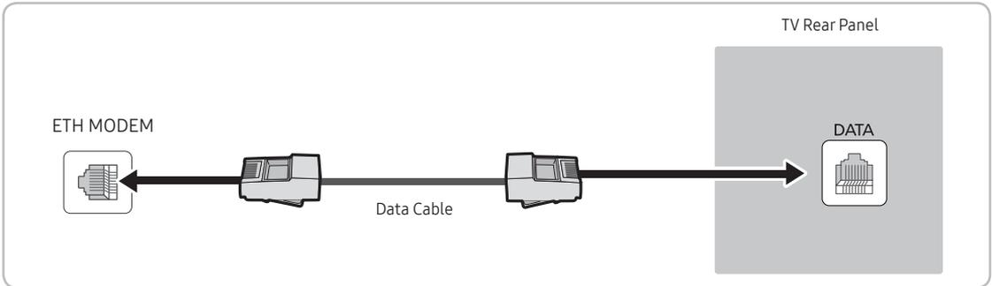
1. Connect the **DATA** jack of the TV to the **ETH MODEM** jack of the STB (SBB) with the Data cable.
