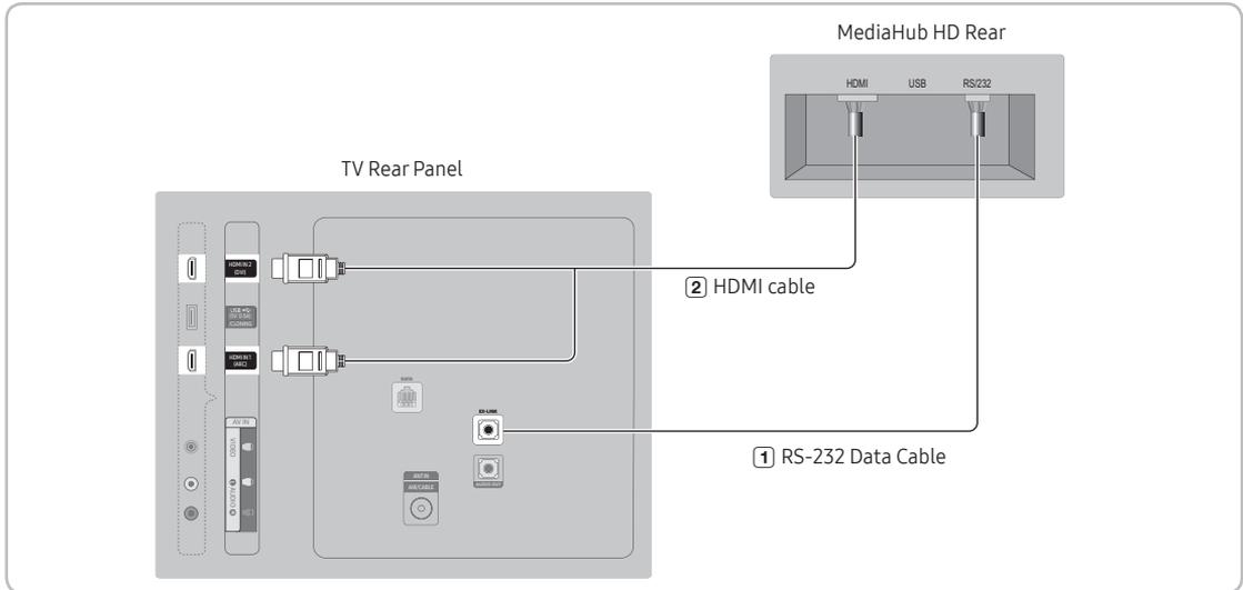
1. Connect the RJP port of the TV and the RS/232 port of the MediaHub HD.
