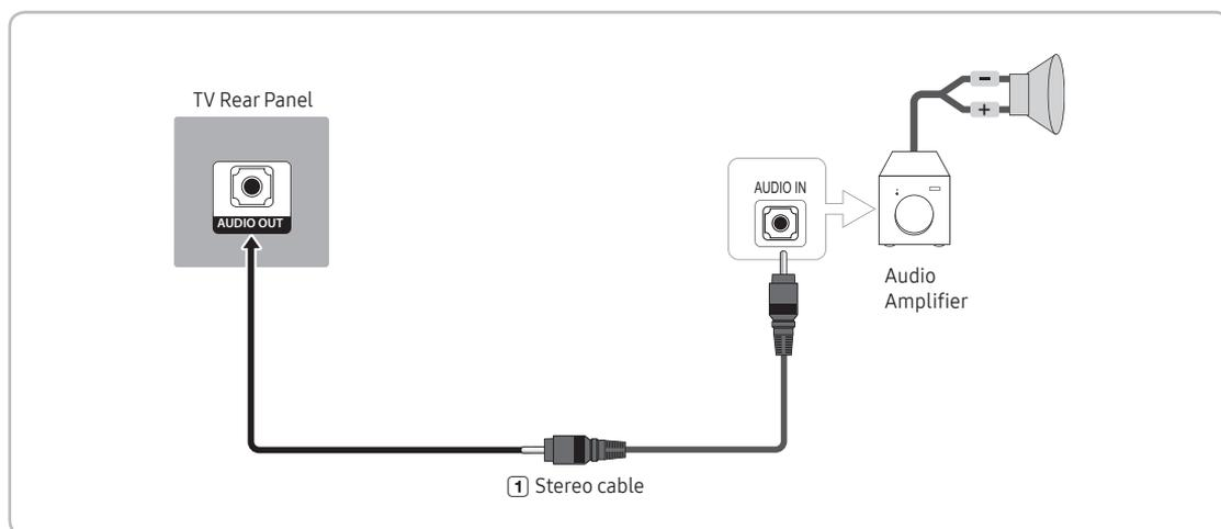
1. Connect the AUDIO OUT port of the TV to the Audio In port of an audio amplifier with a stereo cable. (Stereo cable not provide)
