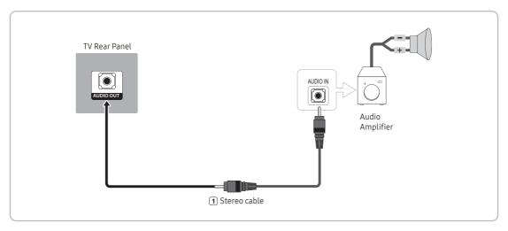
1. Connect the AUDIO OUT port of the TV to the Audio In port of an audio amplifier with a stereo cable. (Stereo cable not provide)
