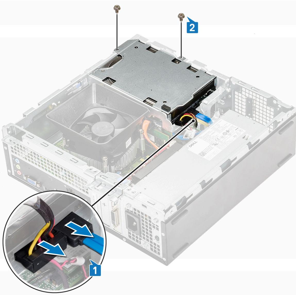
5 Slide the 3.5-inch hard drive chassis and lift it from the system.
