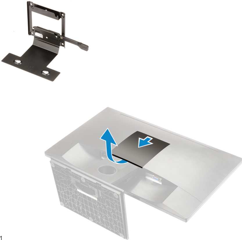
Figure 2. Removing the back cover plates
