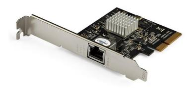
This 4-speed NBASE-T™ PCIe network card offers an inexpensive network upgrade solution, providing access to your network at multiple speeds up to 5G, using your existing Cat5e copper cabling.
