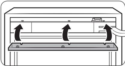
5. Reinsert the ceiling cover, and tighten the screws (x3) to fix the ceiling cover.
