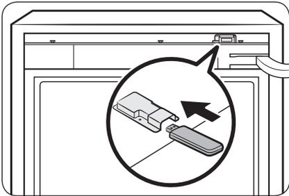
4. Insert the Smart Home Dongle into the dongle port. Make sure the dongle fits.
