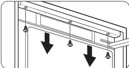
2. Loosen and remove the screws (x3).
