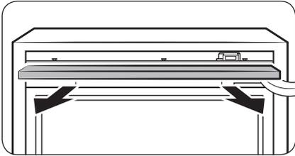
3. Gently pull out the ceiling cover to remove. The dongle port is revealed.
