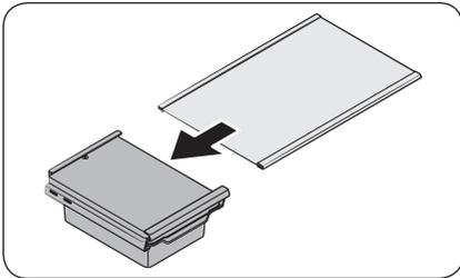
1. Slightly lift up the rear side of the shelf to pull up to the front.
