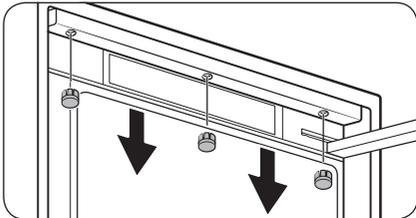
1. Open the fridge door, and use a flat-head screwdriver to remove the 3 screw caps on the ceiling of the main unit.
