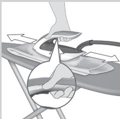
**Note:** in intelligent automatic steam mode, steam comes out automatically when you move the iron and stops when you stop moving the iron. You can still press the steam trigger in this mode to activate the steam when the iron is not moving.
