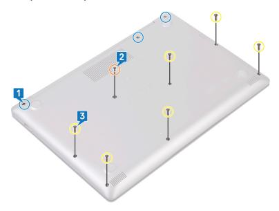
Pry the base cover starting from the top-left corner of the computer base.
