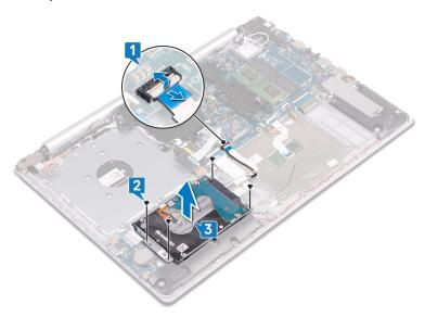
Disconnect the interposer from the hard-drive assembly.
