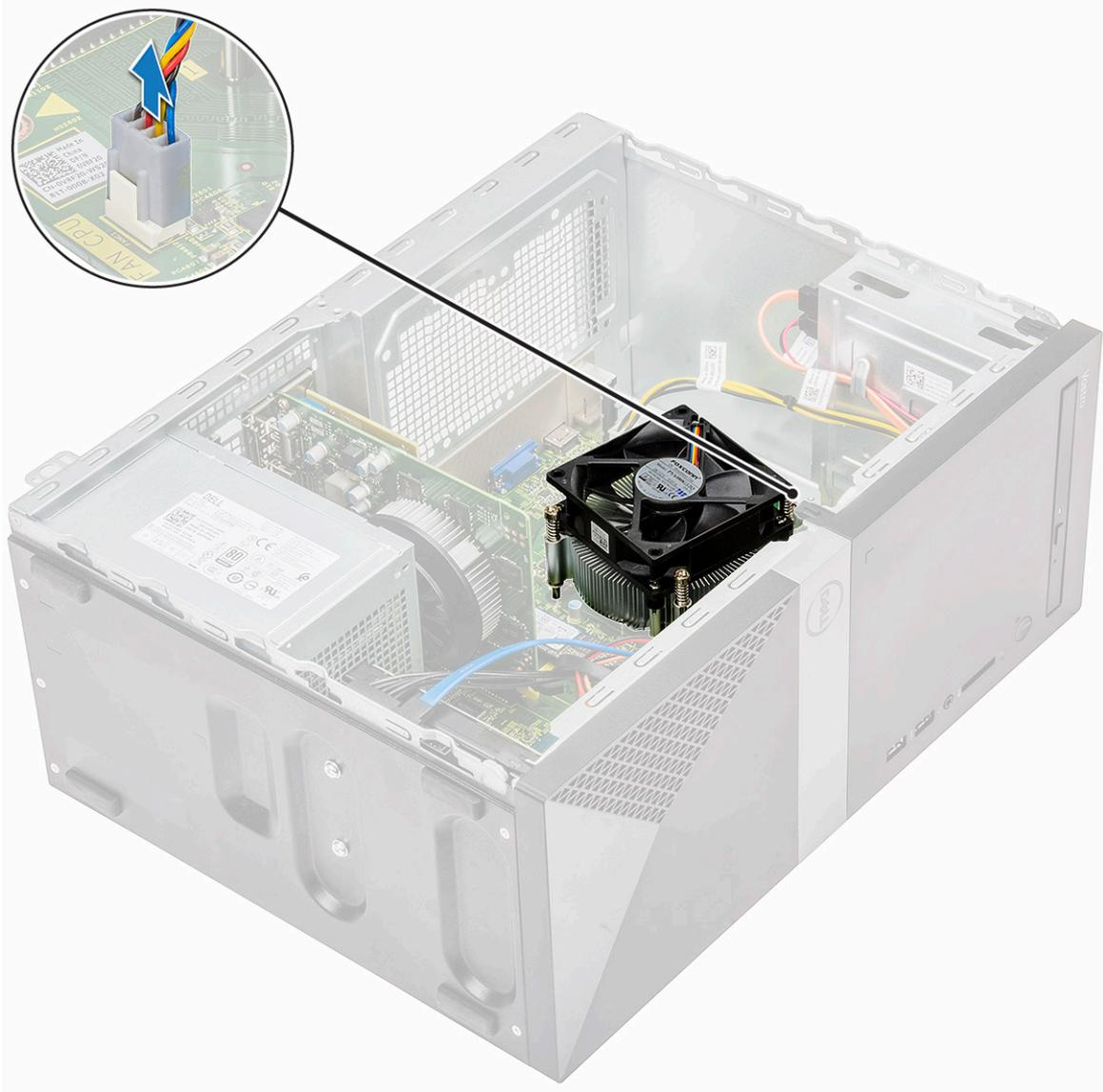
b Loosen the 4 M3 screws in reverse order marked on the system board
