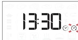
If necessary, turn the knob to set the time you want cooking to end, then press to confirm and start the function. Place the food in the oven and close the door: The function will start automatically after the period of time that has been calculated in order for cooking to finish at the time you have set.
