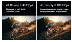
4K Blu-ray format supports more than twice the peak bitrate of 2K Blu-ray which comes in especially handy when watching action movies which have fast paced scenes with a lot of detail. The 100 Mbps peak bitrate of 4K Blu-ray provides enough headroom to store the extra data required to encode high detail fast action scenes and avoid block artifacts.
