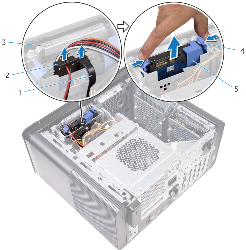
Figure 7. Removing the hard-drive assembly
