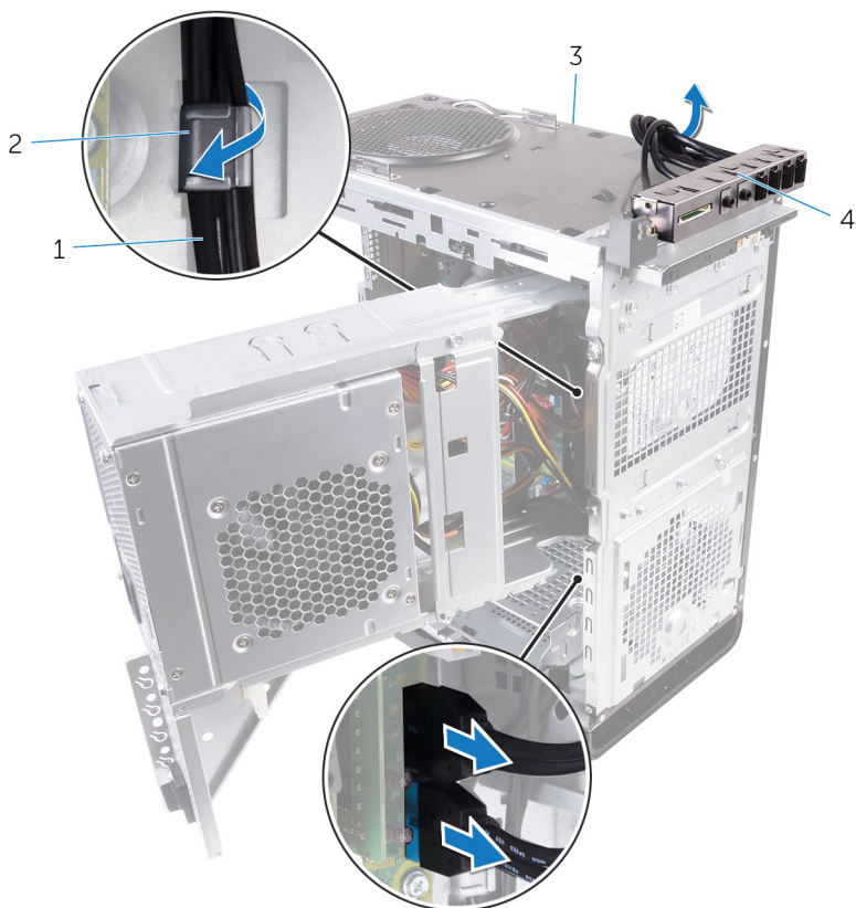
Figure 29. Disconnecting the cables
