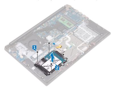
**3** Disconnect the interposer from the hard-drive assembly.
