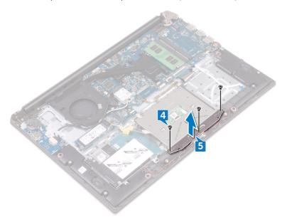
**6** Remove the four screws (M2x2) that secure the touch pad to the palm rest and keyboard assembly.
