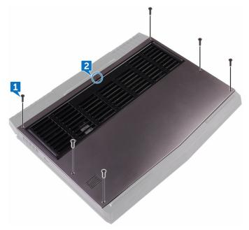
3 Using a plastic scribe, gently pry the base cover to release the tabs on the base cover from the slots on the computer base.
