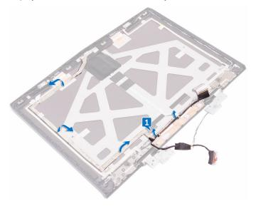
After performing all the above steps, you are left with the display back-cover and antenna assembly.
