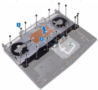
Lift the keyboard at an angle and remove it from the tabs on the palm-rest assembly.
