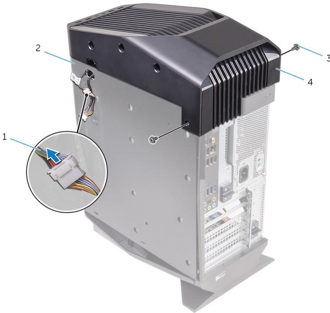
**Figure 9. Removing the top cover**
