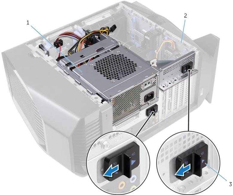
**Figure 2. Sliding the power-supply unit cage release latches**
