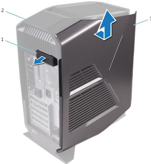
**Figure 1. Removing the left-side cover**
