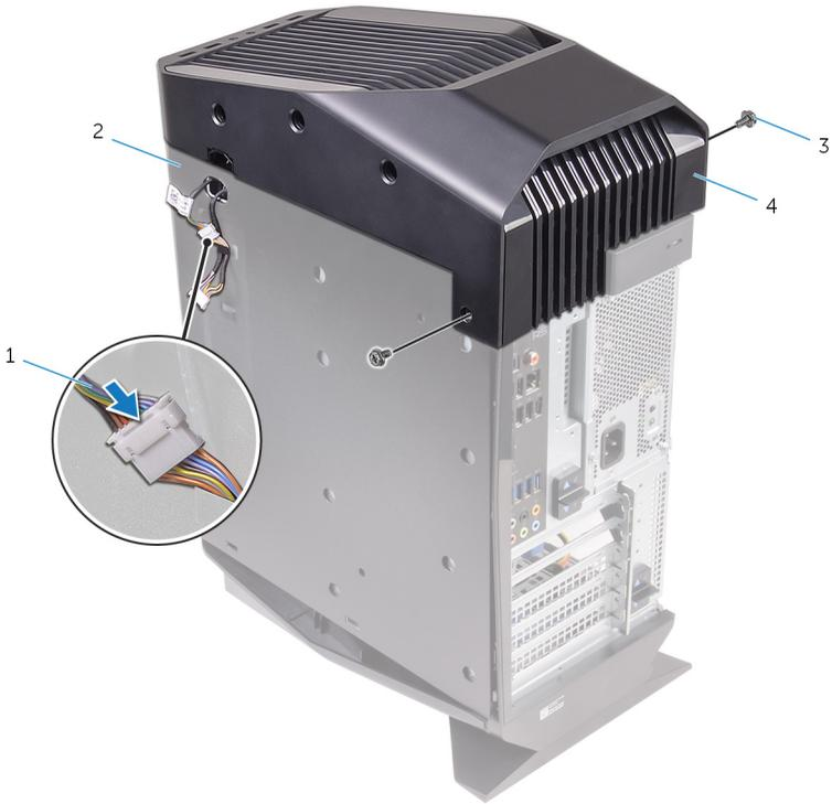
**Figure 15. Replacing the top cover**
