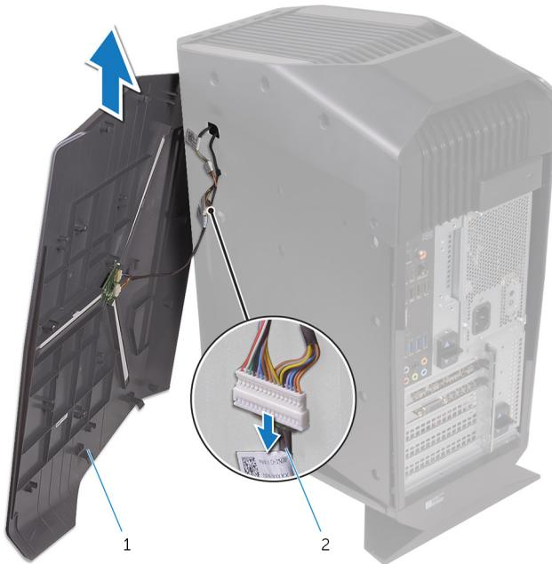
**Figure 8. Removing the right-side cover**
