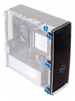
**3** Rotate and pull the front bezel away from the front of the computer to release the front bezel tabs from the front panel slots.
