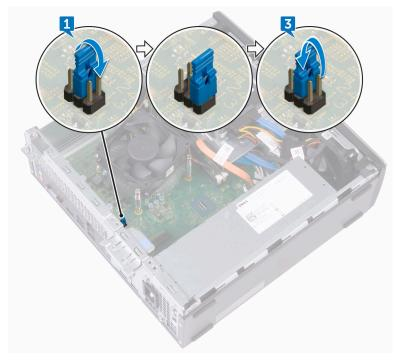
**3** Wait for 5 seconds and then replace the jumper plug to its original location.
