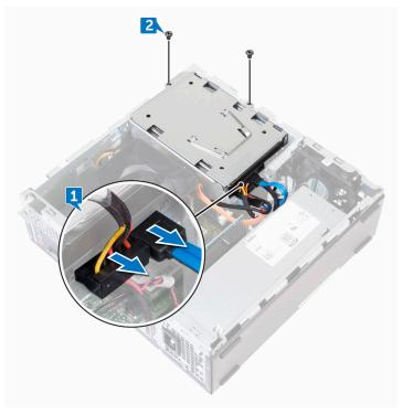
**3** Using the pull-tab, slide the hard-drive assembly toward the inside of the computer and lift it off the drive cage.
