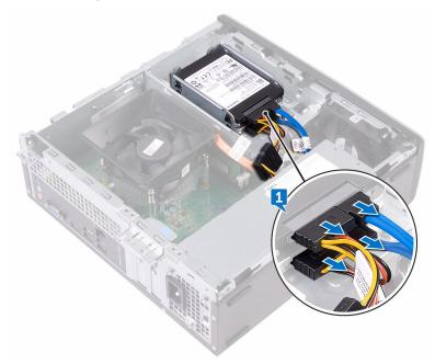
**2** Remove the screw (#6-32xL3.6) that secures the hard-drive assembly to the drive cage.
