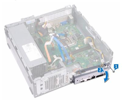
2 Swivel open the front I/O bracket from the Chassis.
