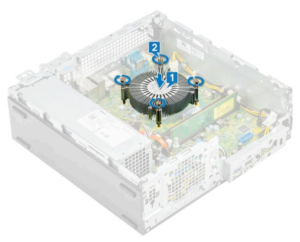
Place the heat sink cover onto the heat sink.
