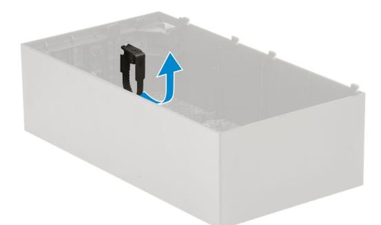
4 Lift the tab [1] to release and pull the cable tie from the slot on the cable release latch [2].
