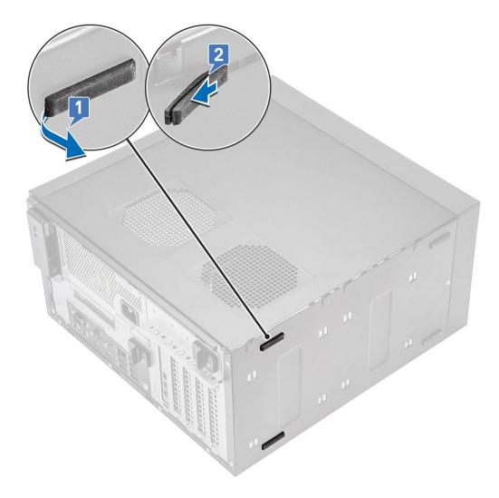
Figure 5. Rear rubber feet removal
