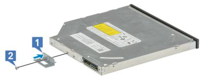
2 Slide the optical drive into the drive bay from the front of the computer until it is secured.
