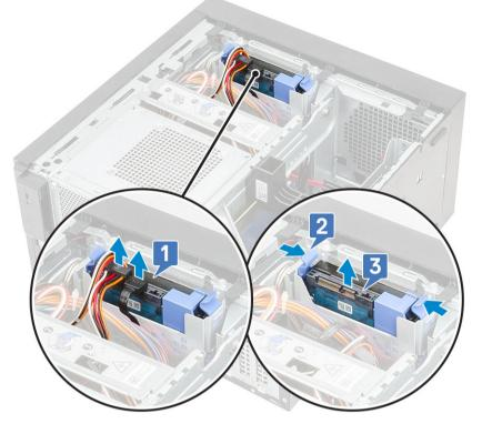
5 Flex the hard drive bracket and lift the hard drive from the hard drive bracket.
