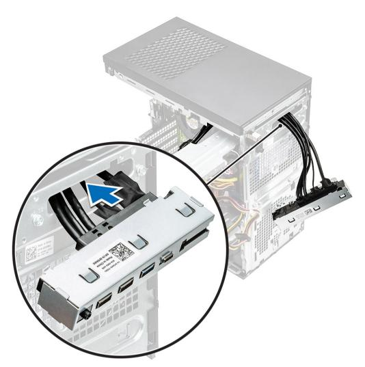
2 Insert the IO-panel tabs into the slots on the system [1] and tilt the IO panel to secure it to the system [2].
