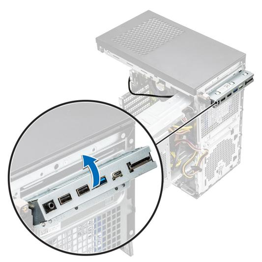
7 Pull the IO panel along with the cables to remove it from the IO panel slot on the chassis.
