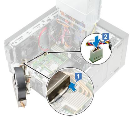
2 Place the heat-sink assembly over the processor.
