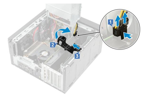
7 Push the card retention latch away from the card [1] and lift the graphics card out of the computer [2].
