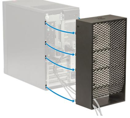
11 Open the tab and unroute the cables from cable tie [1], disconnect the cables from the ports on the system [2]. Remove the cables from the slot of the cable cover [3].
