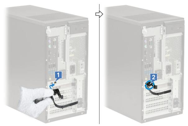
6 Route the cables through the slot of the cable cover [1], and connect them to their respective ports on the system [2]. Secure the cable with the cable tie and lock the tab in place [3].
