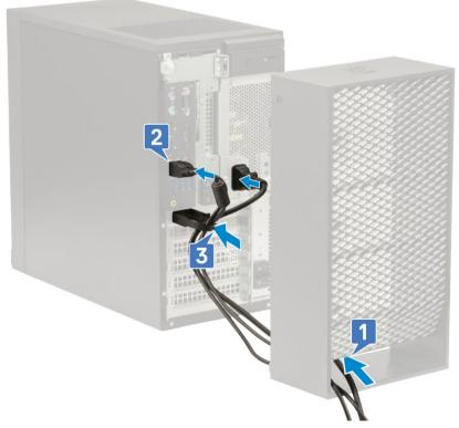
7 Align the plastic hooks of the cable cover to the slots on the system .
