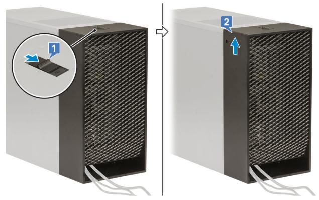
10 Pull the cable cover to release it from the chassis.
