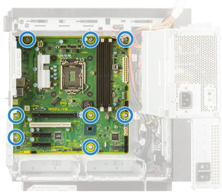
7 Lift the system board at an angle and remove it from the computer.
