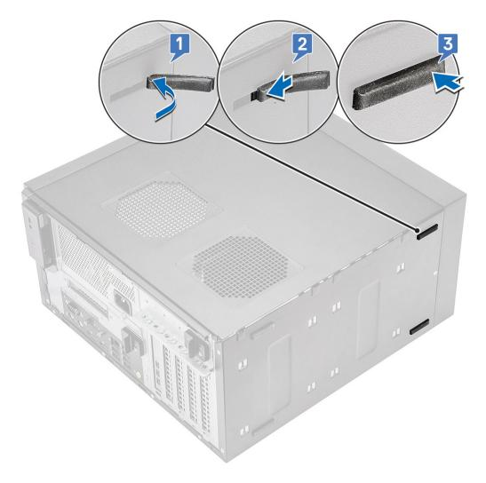
Figure 6. Front rubber feet installation
