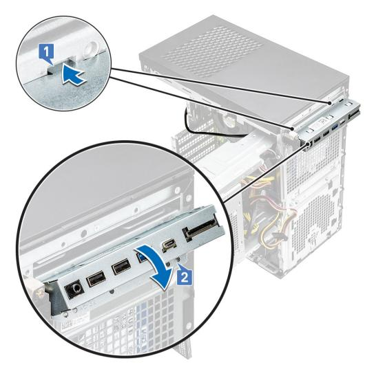
3 Replace the #6-32x1/4" screw to secure the IO panel to the system.
