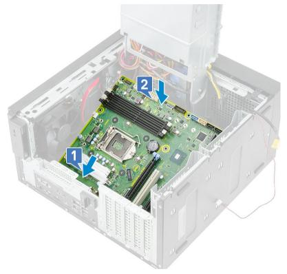
2 Replace the 8 #6-32x1/4" screws that secure the system board to the chassis.
