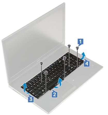
g Slide and remove the keyboard from the system.
