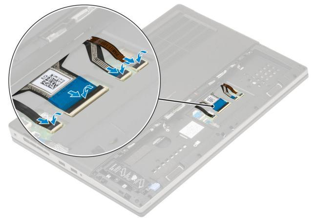
(i) NOTE: Ensure that you fold the keyboard data cable in perfect alignment.
