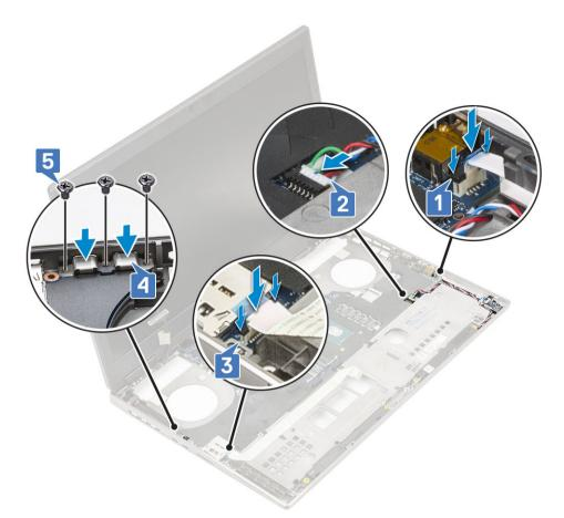
f Connect the power connector cable and battery cable to the connectors on the system board [1, 2].
