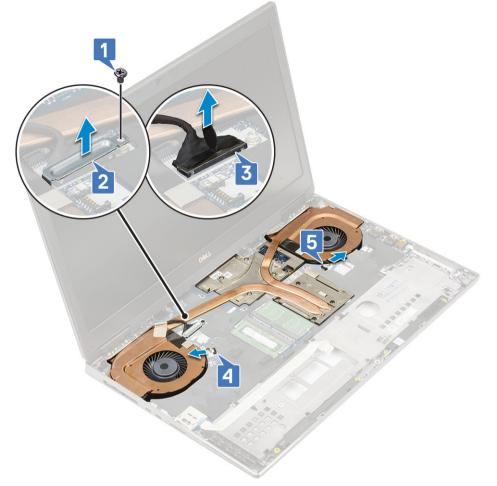
f Loosen the 8 captive screws that secure the heat sink assembly to the system board [1].
