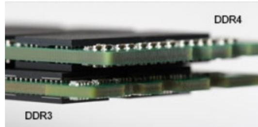
**Figure 2. Thickness difference**
