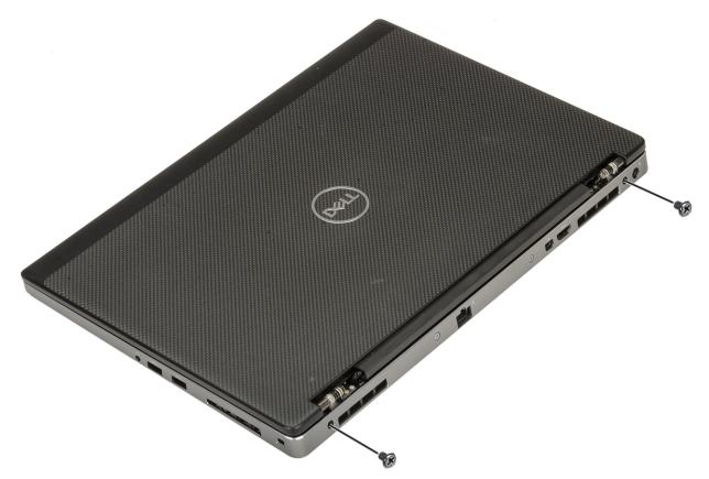
h Route all the wireless antenna cables to the routing channels at the bottom of the system and next to the hinge caps [1].i Replace the 2 (M2.5x4.0) screws at the bottom of the system to secure the display assembly in place [2].
