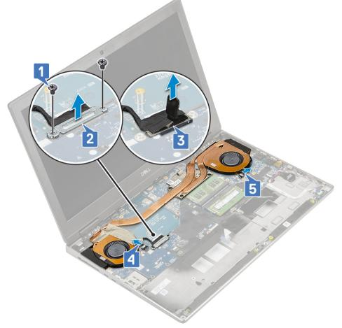
f Loosen the 4 captive screws that secure the heat sink assembly to the system board [1].
