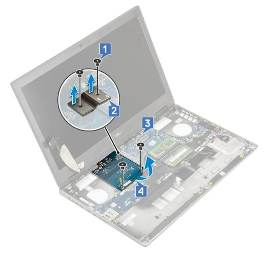
INOTE: The above procedures are for UMA graphics card. Systems shipped with UMA GPU card do not have GPU power cable. However, for discrete models shipped with either a 128 MB or 256 MB VRAM GPU card, you need to disconnect the GPU power cable before removing the GPU card.
