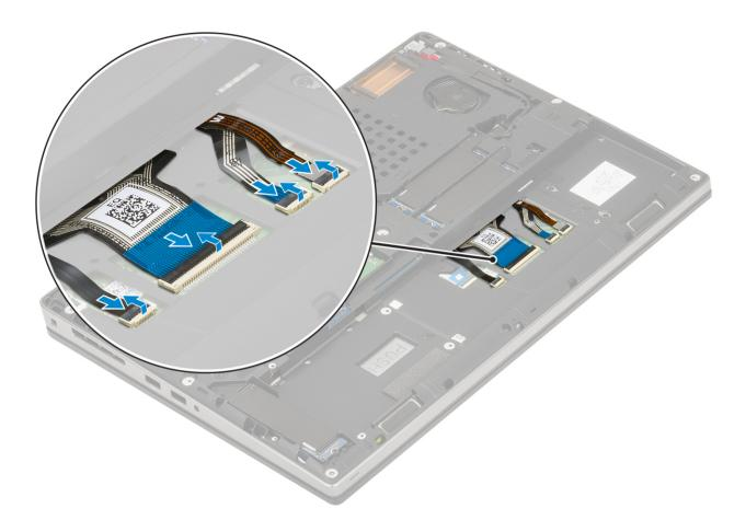
(i) NOTE: Ensure that you fold the keyboard data cable in perfect alignment.
