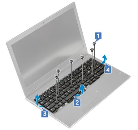
g Slide and remove the keyboard from the system.
