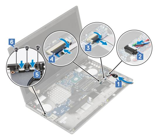
f Connect the power connector cable to the connector on the system board [1, 2].
