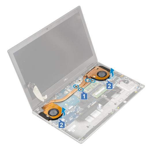
h Slide and remove the heat sink assembly from the system.
