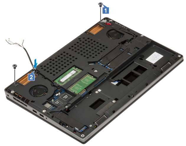
c Remove the 2 (M2.5x6.0) screws at the rear of the system that secures the display assembly in place.
