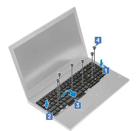
d Align the keyboard lattice to its position on the keyboard and ensure that the keyboard lattice clicks into its place.
