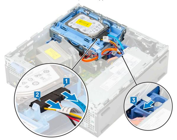
c Unroute the hard drive cables [1] and optical drive cables [2] through the retention clip and HDD-ODD release tab respectively.
