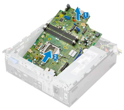
3 Replace the 5 screws that secure the system board to the system [1], the single (M3x5) screw [2], and the single (#6-32) screw [3].
