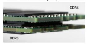
Figure 2. Thickness difference
