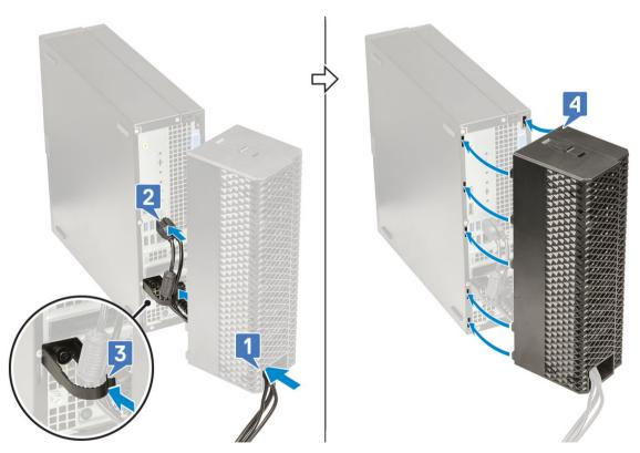
Gently press down on the cable cover until it clicks into place (1). Slide the latch towards the chassis (2) to lock the cable cover in place.
