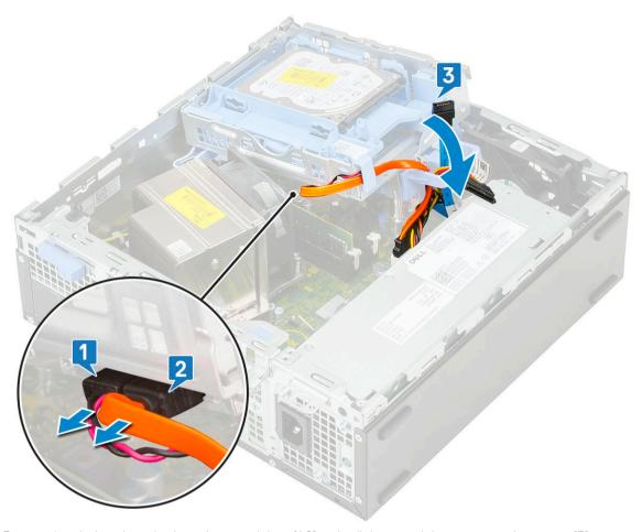
e Press and push the release latch on the optical drive [1,2] and pull the optical drive out from the system [3].
