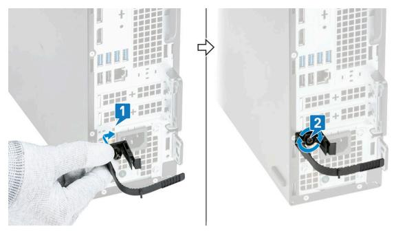
Route the cables through the slot of the cable cover [1], and connect them to their respective ports on the system (2). Secure the cable with the cable tie and lock the tab in place [3]. Align the plastic hooks of the cable cover to the slots on the system [4].
