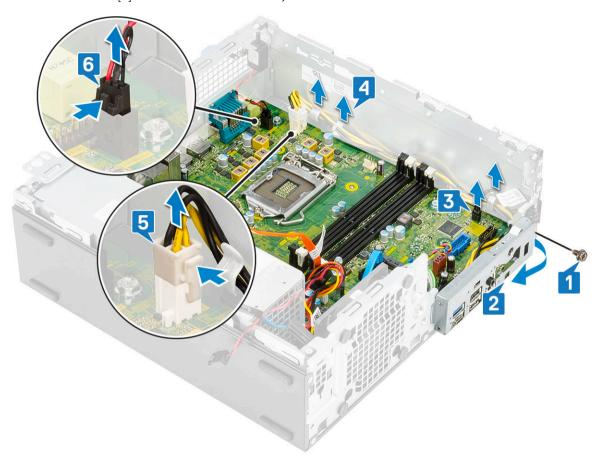
Disconnect the intrusion switch cable [1], PSU power cable [2], data cable [3], system fan cable [4], SATA cable [5], SATA power cable [6]
