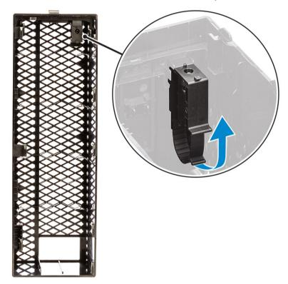
3 Lift the tab [1], to release and pull the cable tie from the slot on the cable release latch [2].
