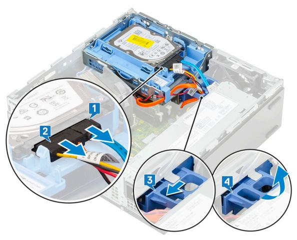
d Disconnect the optical drive data cable and optical drive power cable from the connectors on the optical drive [1, 2] and lower the hard drive and optical module until it is seated [3].
