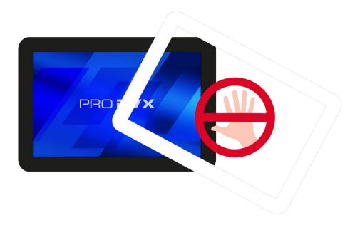
8. Slowly lower the uncovered adhesive side onto your screen cover while carefully aligning it with the sides, bottom and active area of the LCD screen of your device. If it does not align perfectly, gently lift immediately and adjust until you are satisfied.
