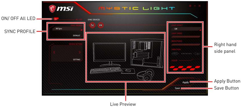
• **ON/OFF ALL LED** - By toggling Off/On here, you disable/enable all the LED on supported gaming gear, memory, graphics card and motherboard etc.
