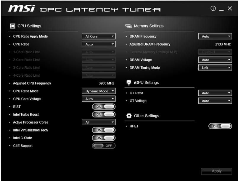
Install and open the DPC LATENCY TUNER control panel, it allows you to set CPU, memory and iGPU settings. After then you must click the **Apply** button to restart the computer and apply your changes.
