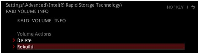
5. Select the **Rebuild** item and press **Enter** key to rebuild the new hard drive.
