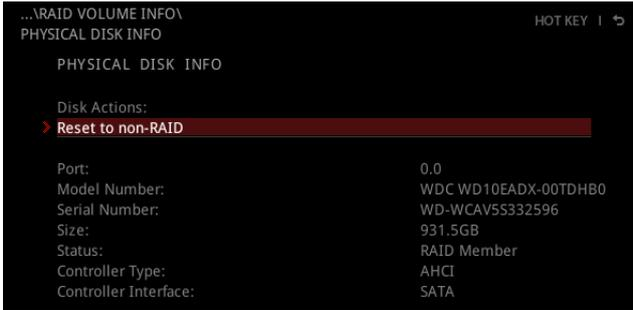
4. Select **Reset to non-RAID** item and press **Enter** to delete the RAID volume and remove any RAID structures from the drives. The following screen appears:
