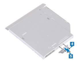
6 Pull the optical-drive bezel carefully to remove it from the optical drive.
