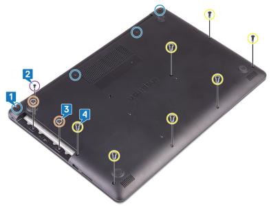
**5** Pry the base cover starting from the top-left corner of the computer base.
