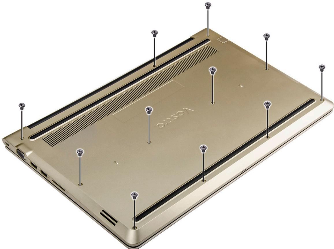
**Figure 5. Removing screws**
