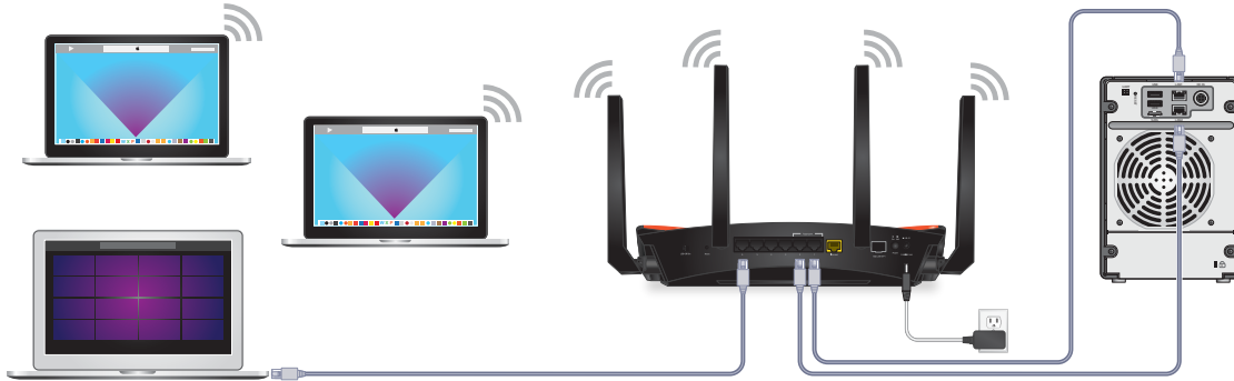
Figure 7. Ethernet port aggregation
