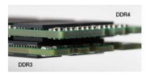
Figure 2. Thickness difference
