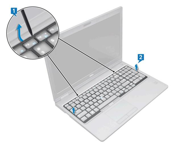
ONOTE: Use a plastic scribe to pry the keyboard lattice from the pry points and move around the lattice for removal.
