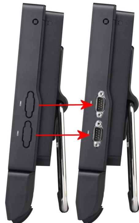
Shuttle XPC all-in-one P20U/P22U before and after the installation of PCP21
