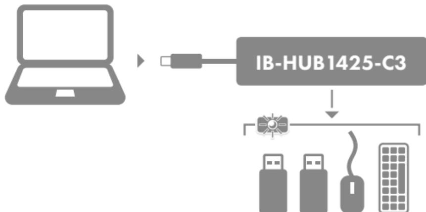
1. Plug the IB-HUB1425-C3 into the Type-C™ port of your host computer.
