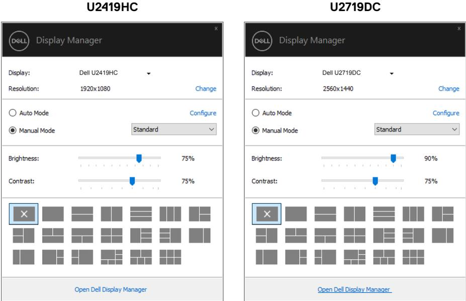
The **Quick Settings** dialog box also provides access to Dell Display Manager's advanced user interface that is used to adjust basic functions, configure auto mode and access other features.
