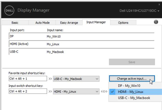
**NOTE:** DDM communicates with your monitor even when the monitor is displaying video from another computer. You can install DDM on the computer you frequently use and control input switching from it. You may also install DDM on other computers connected to the monitor.
