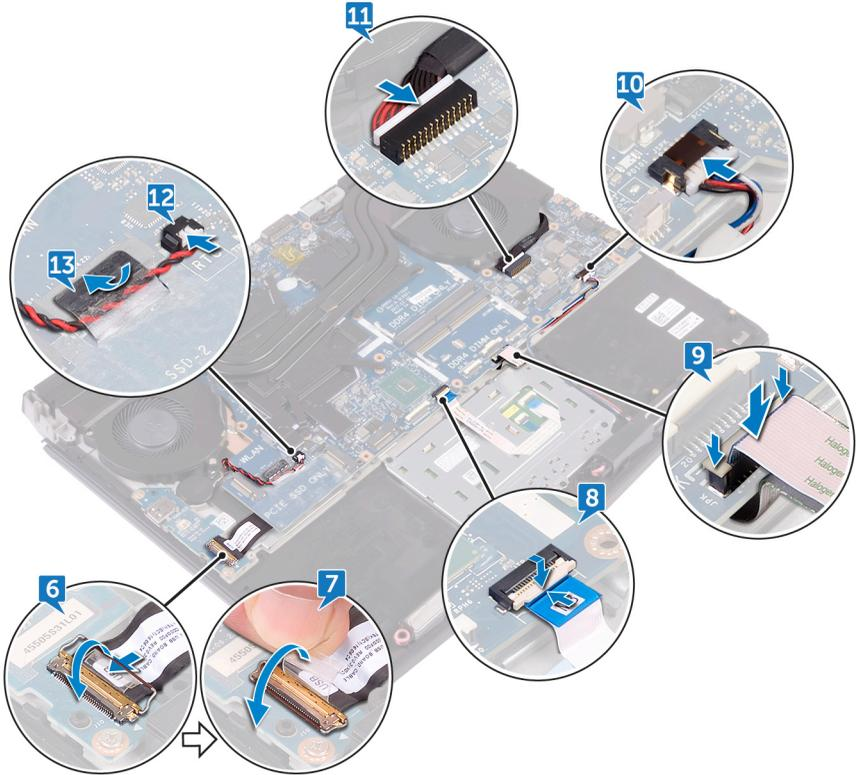
**14** Connect the keyboard cable (optional) to the system board.
