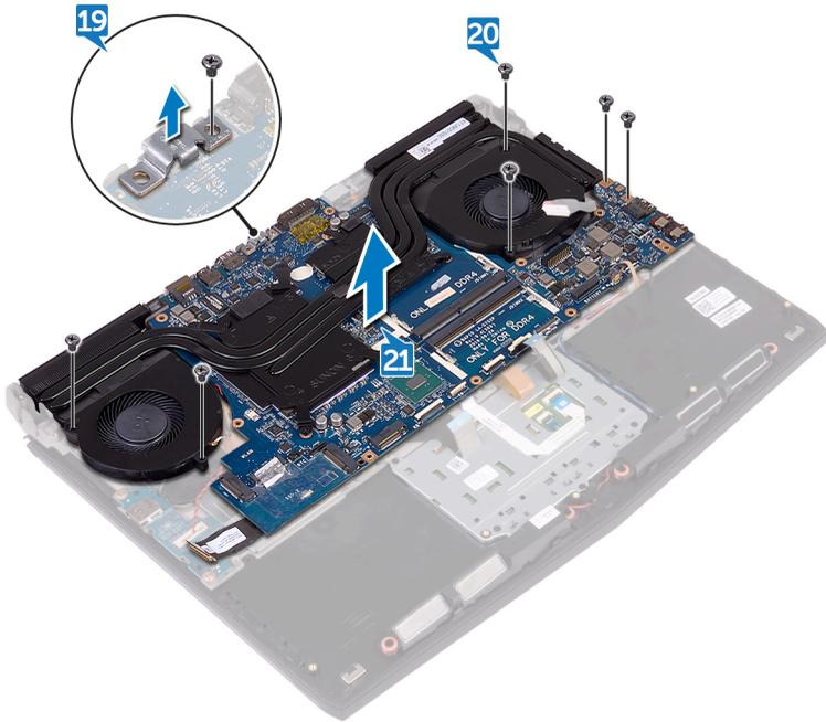
**22** Remove the [heat-sink assembly](#).
