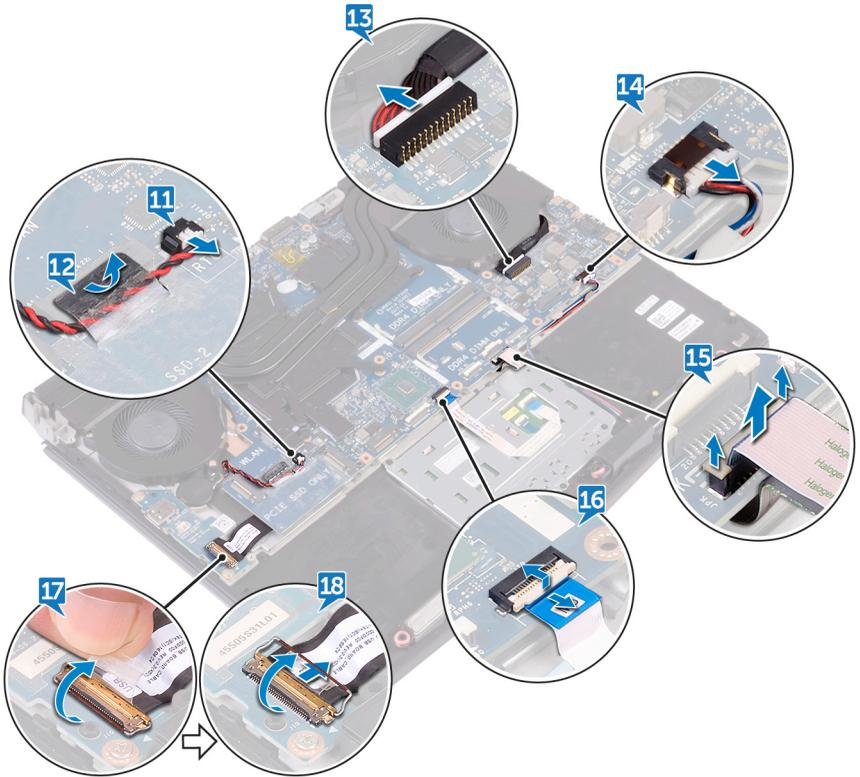
**NOTE:** Note the orientation of the USB Type-C port bracket before removing it from the system board.
