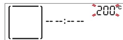
When the value flashes on the display, turn the *adjustment knob* to change it, then press  $\checkmark$  to confirm and continue to alter the settings that follow (if possible).
