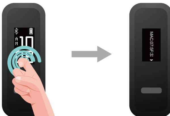
**Method 2:** View the Bluetooth name and MAC address on the back of your band body. The Bluetooth name of your band is **HUAWEI Band 3e-XXX**, while the band's MAC address is in 12 alphanumeric characters next to **MAC:** .
