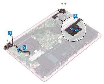
4 Lift the palm-rest and keyboard assembly at an angle.
