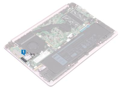
2 Remove the screw (M2x5) that secures the wireless-card bracket to the I/O board.
