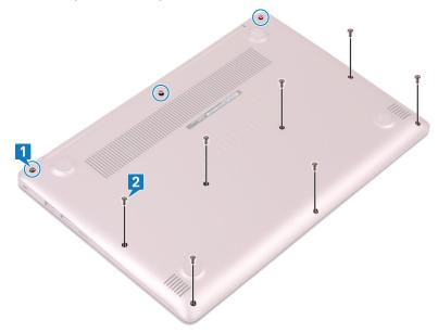
**3** Pry the base cover starting from the top-left corner of the computer base.
