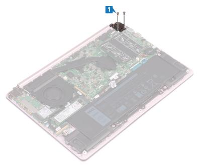
2 Lift the palm-rest and keyboard assembly at an angle to lift up the right hinge.
