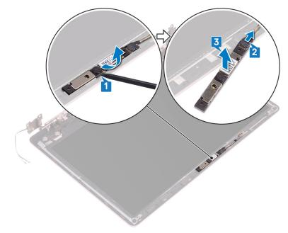
**3** Lift the camera module from the display back-cover and antenna assembly.
