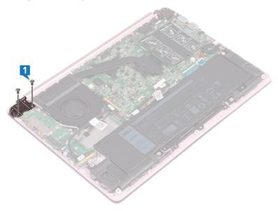
2 Lift the palm-rest and keyboard assembly at an angle to lift up the left hinge.
