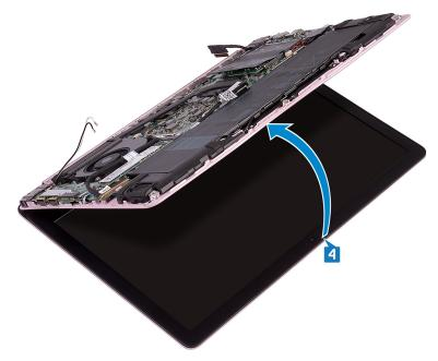
5 Slide and remove the palm-rest and keyboard assembly off the display assembly.
