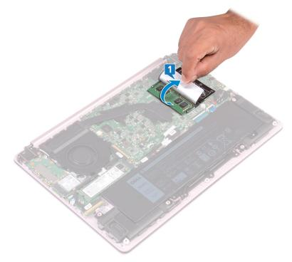
**2** Use your fingertips to carefully spread apart the securing-clips on each end of the memory-module slot until the memory module pops up.
