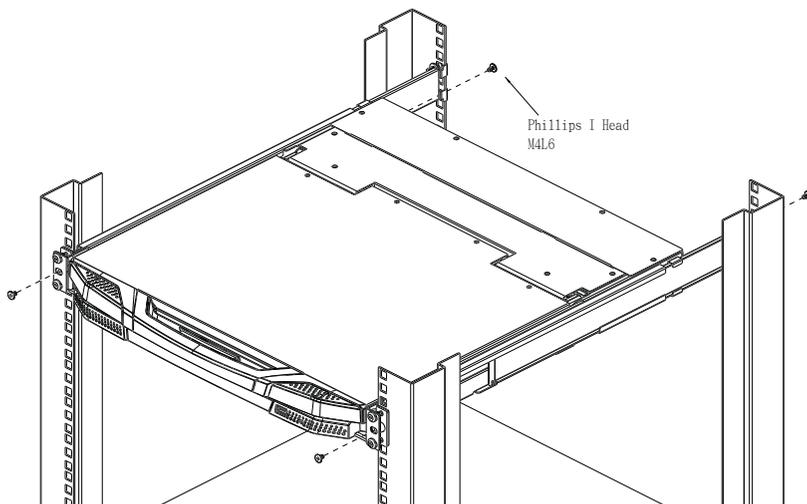
5. Slide the CL3800 / CL3700 / CL3100 open and closed a couple of times to be sure that it is properly aligned and operating smoothly. (See *Opening / Closing the Console*, page 23, for opening and closing procedures.)
