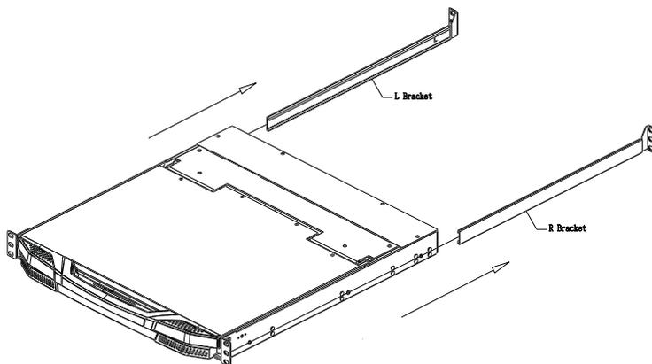
2. Attach the left and right *easy-installation* mounting rails to the inside of the rack. The flange that supports the CL3800 / CL3700 / CL3100 will be to the inside.
