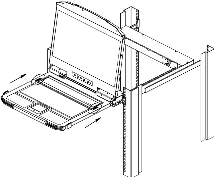
6. Slide the keyboard in until it's completely inserted into the rack.
