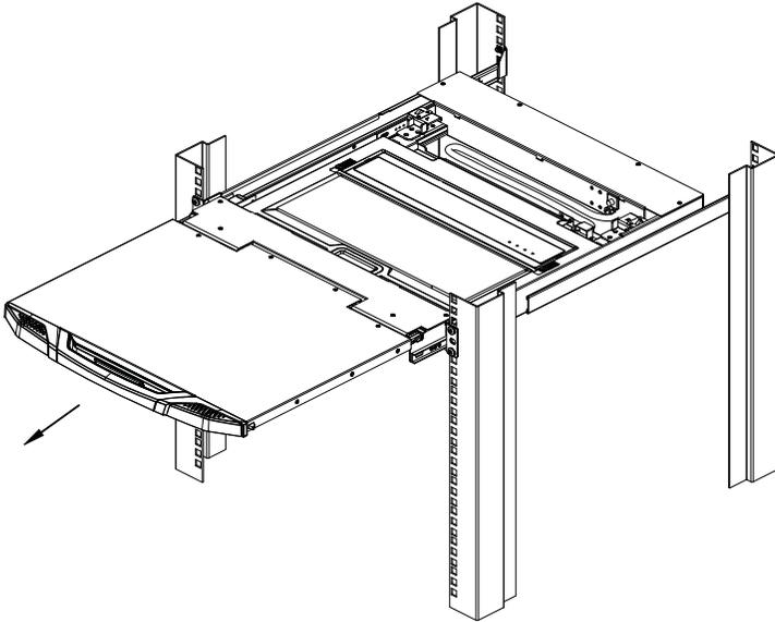
3. Raise the top panel all the way back to expose the LCD screen.
