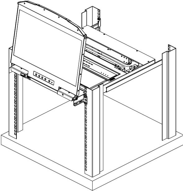
7. To close the LCD screen, lower the panel module until it lies flat and slide it back in.
