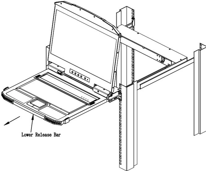
5. To independently retract the keyboard into the rack, slide both Keyboard Module Releases and push the keyboard module all the way in.
