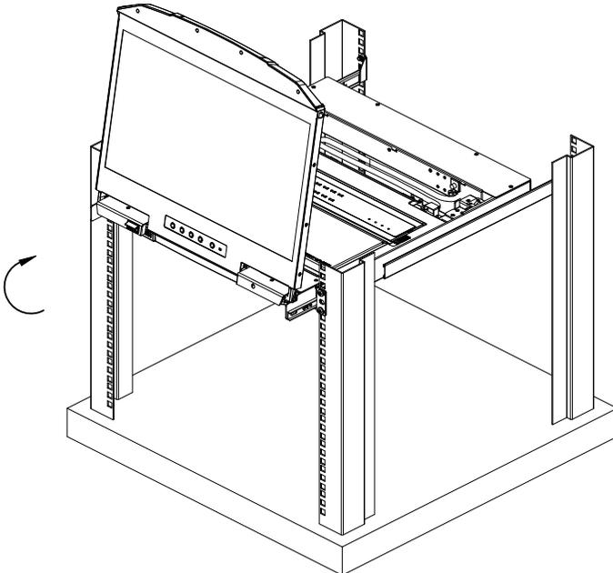
4. Use the Lower Release Bar handle to pull the keyboard module straight out unit it clicks in place.
