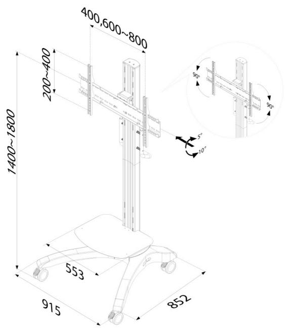
Neomounts Measuring unit: mm
