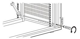
2. Remove the rods from the enclosure.
